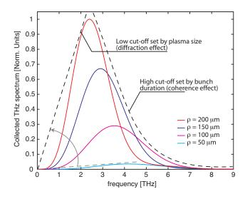
Figure 3: Predicted spectra (0.5 nC,  $\sigma_z = 15 \ \mu\text{m}$ ,  $E_c = 45 \ \text{MeV}$ ) of CTR collected by a 6-inch OAP (19° off-axis) for different plasma transverse boundary sizes ( $\rho$ ). The amount of emitted energy is strongly affected by the transverse boundary size of the emitting region.
